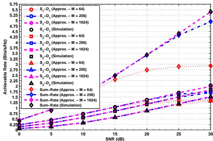
Fig. 2. Achievable Rate: Approximation vs. Simulation - EPA
