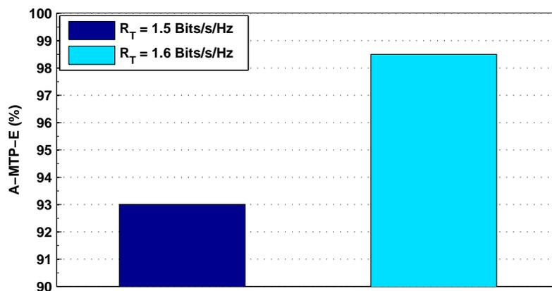
Fig. 9. Average Minimum Total Power Efficiency - SNR = 30 dB and  $M = 1024$
